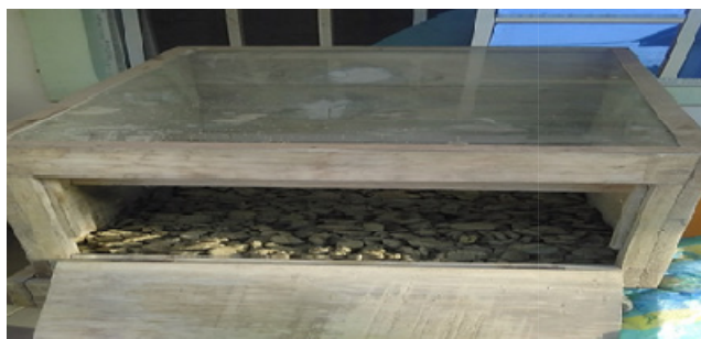
Plate 1: Seed meals in Solar cabinet dryer
